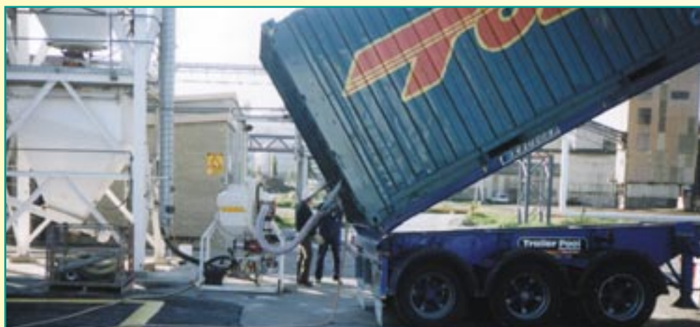
A Toll container at a 45 degree angle attached to the new bulk conveying system developed by Toll SPD.
